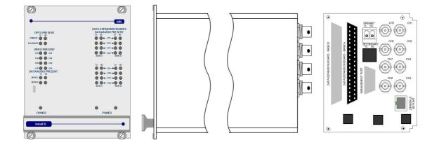
The **AMG4788AER-SF** is a rackmount eight channel video receive unit designed to receive 8 video signals and transmit and receive up to 8 data or audio signals plus full duplex 100BaseT Ethernet connectivity over one singlemode fibre. The 8 data/audio channel interfaces, whether RS232, RS422, RS485, 20mA, TTL, Contact Closure, Lonworks or Audio, are defined at manufacture by the addition of daughter boards fitted onto the Data Expansion Board A.
